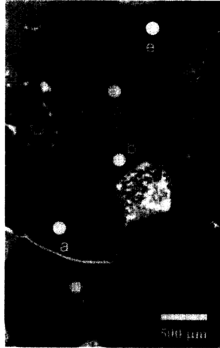
Fig. 3. Microstructure of pure Zn, which was electropolished in 10 % HClO 4 + 90 % CH 3 COOH solution. The small circles indicate the points where the electrochemical tests were performed.
