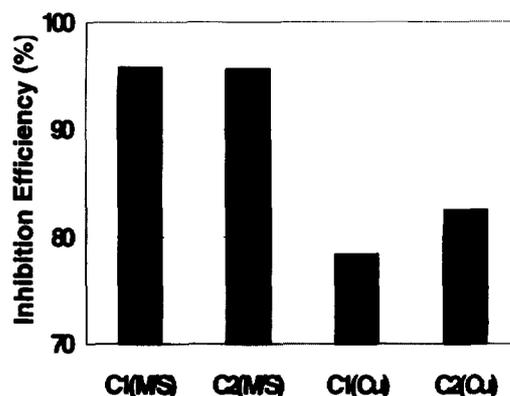
Fig. 5. Inhibition efficiency of triple inhibitor combinations for mild steel and copper in LiBr solution
