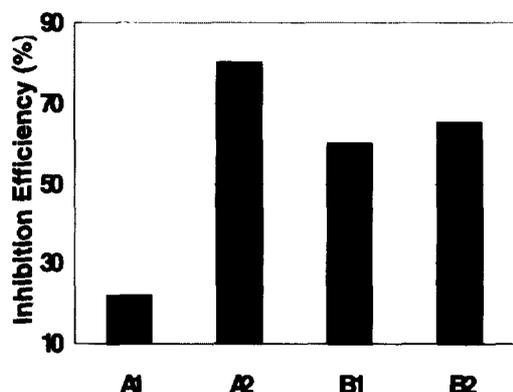
Fig. 4. Inhibition efficiency of double inhibitor combinations for copper in LiBr solution
