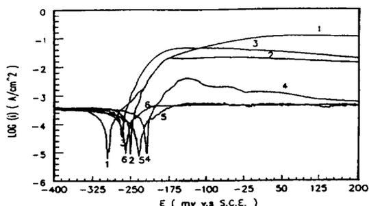
Fig. 1. Anodic polarization curves of mild steel in LiBr solution with or without various inhibitors [3] (1 : Blank, 2 : Li<sub>2</sub>CrO<sub>4</sub> only, 3 : BTA only, 4 : LiOH only, 5 : BTA + LiOH + Li<sub>2</sub>CrO<sub>4</sub>, 6 : LiOH + Li<sub>2</sub>CrO<sub>4</sub>)
