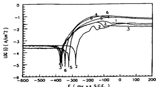
Fig. 2. Anodic polarization curves of copper in LiBr solution with or without various inhibitors [3] (1 : Blank, 2 : Li<sub>2</sub>CrO<sub>4</sub> only, 3 : BTA only, 4 : LiOH only, 5 : BTA + LiOH + Li<sub>2</sub>CrO<sub>4</sub>, 6 : LiOH + Li<sub>2</sub>CrO<sub>4</sub>)
