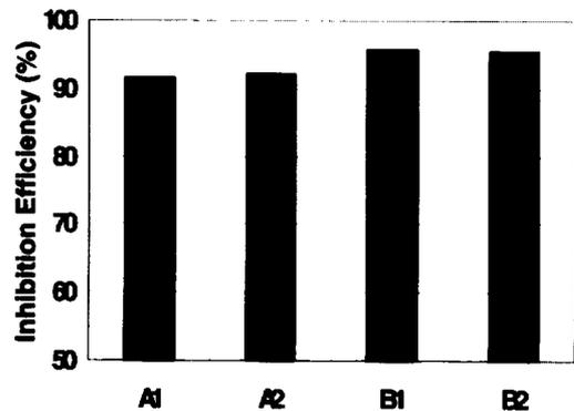
Fig. 3. Inhibition efficiency of double inhibitor combinations for mild steel in LiBr solution
