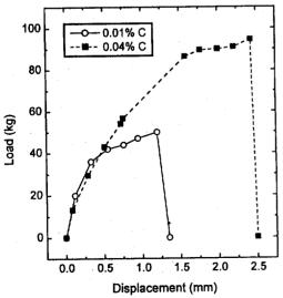
Fig. 12. Load-displacement curves during SSRT in primary water at 360°C.
