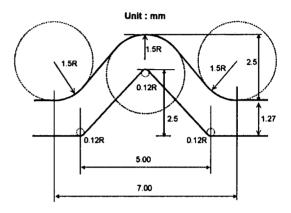
Fig. 3. Dimension of hump press die.
