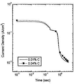
Fig. 8. Repassivation behavior measured by a potential pulse from -1,000 mV $_{\rm Ni}$  to +200 mV $_{\rm Ni}$  in 10% NaOH at 315°C.
