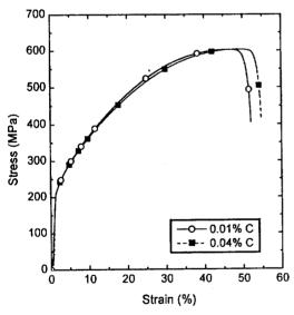
Fig. 1. Stress strain curves in air at room temperature.
