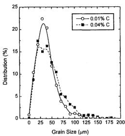
Fig. 6. Grain size distribution measured by an image analyzer.
