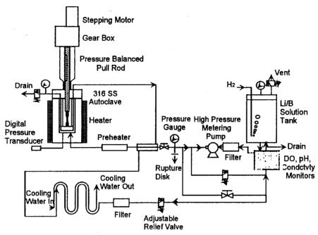
Fig. 4. Schematic of loop system for SSRT under sim- ulated primary water condition.
