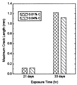
Fig. 9. Evolution of maximum crack depth in 10% NaOH at 315°C.
