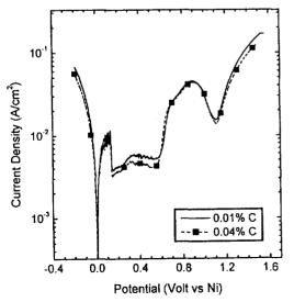
Fig. 7. Polarization curves in 10% NaOH at 315°C.
