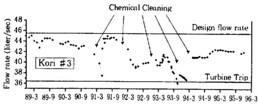
Fig. 1. Stator Flow Rate History at a Nuclear Power Plant during 1989~1996.
