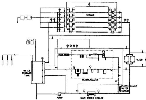
Fig. 4. Schematic of Stator Simulation Loop System.
