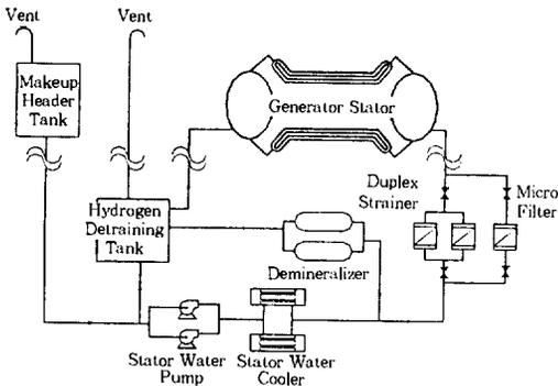
Fig. 2. Generator Stator Water System Schematic for the Nuclear Power Plant.
