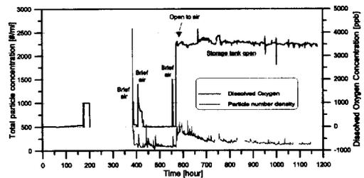
Fig. 8. Water-borne Particle Number Density and Dissolved Oxygen Concentration with Time during Hydrogenated Water Experiment (from 0 to 200 hr) and Aerated Water Experiment (from 450 to 1,150 hr).
