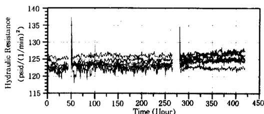
Fig. 5. Strand Hydraulic Resistance during the Final 420 Hour Period of 200 ppb Oxygen Water Experiment.
