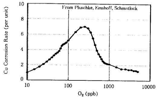
Fig. 3. Corrosion Rate of Copper Determined by 10,000 Hour Test in Neutral Stator Water Environment(reproduced from Ref. 2).
