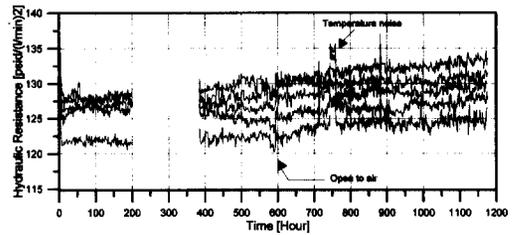
Fig. 7. Strand Hydraulic Resistance with Time during Hydrogenated Water Experiment (from 0 to 200 hr) and Aerated Water Experiment (from 450 to 1,150 hr).
