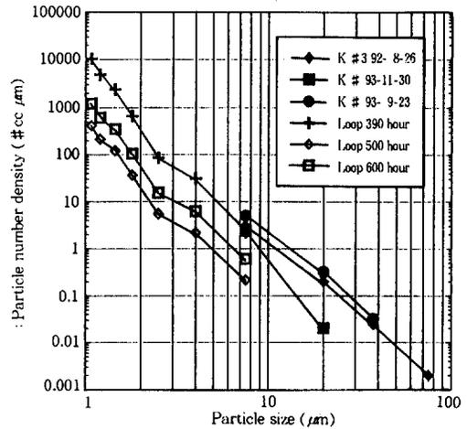
Fig. 11. Comparison of Water-borne Particle Number Density between Loop Experiment with Aerated Water and the Nuclear Power Plant during Flow Degradation Period.
