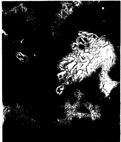
Fig. 7. Corrosion morphology of AZ91-T6.
