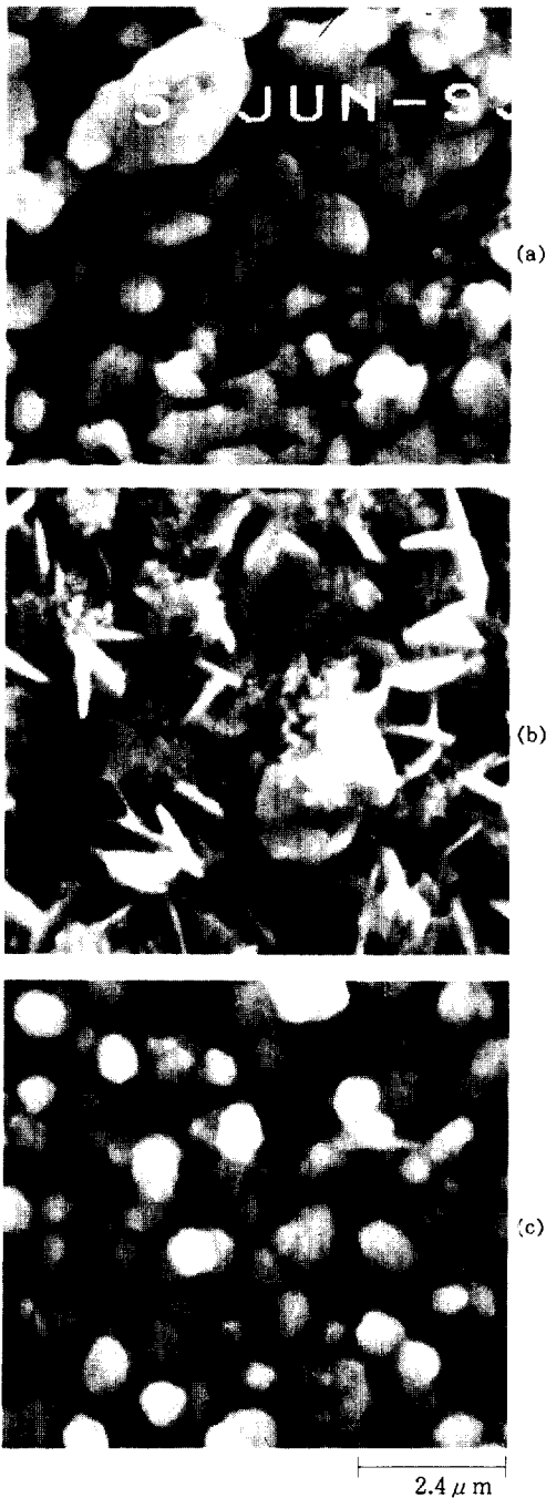
Fig. 6. SEM micrographs of Zn electrodeposit on Pb substrate (solution : 9.08m KOH + 0.63m ZnO + 2.54 \times 10^{-4} m PbO, potential window : -1.5V_{\text{Hg}/\text{HgO}} \sim -0.8V_{\text{Hg}/\text{HgO}} , magnification 5000 \times , v=20 mV/s) (a) 1cycle (b) 3cycles (c) 6cycles
