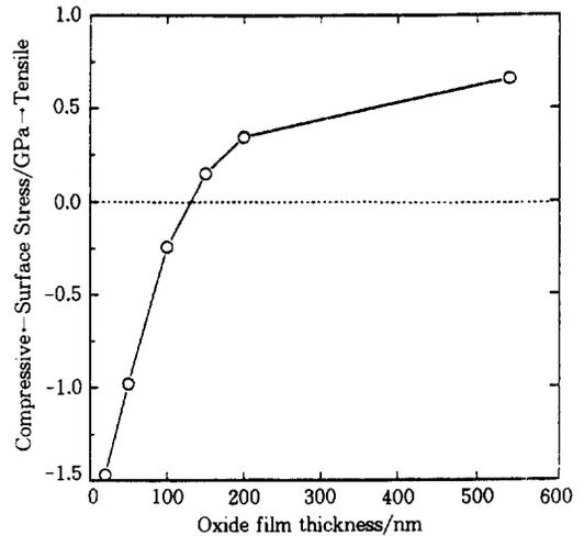
Fig. 4. Change in surface stress with oxide film thickness for an anodic oxidation of aluminium strip specimen at an applied current density of  $3.3\text{mA cm}^{-2}$  in ammonium borate solution (pH=9.7) taken from Bradhurst and Leach.<sup>5)</sup> Dotted line indicates the zero position of deflection.
