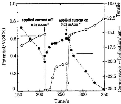
Fig. 1. Responses of potential(○) and deflection (●) to current interruption during anodic oxidation of tungsten strip specimen at an applied current density of 0.02mA cm<sup>-2</sup>.
