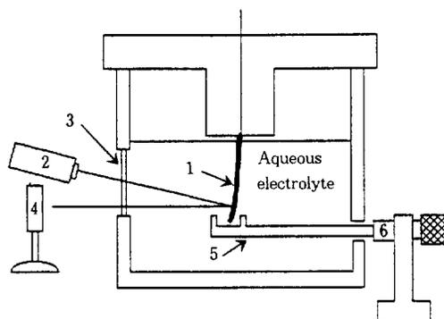
Fig. 3. A beam deflection apparatus used to measure stress development on the surface of metal : 1, specimen; 2, laser source; 3, flat window; 4, photocell; 5, stainless steel rod; 6, micrometer.
