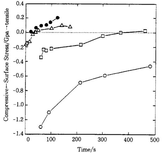
Fig. 5. Changes in surface stresses with time for anodic oxidation of tungsten strip specimen at applied current densities of : ○ , 0.02mA cm<sup>-2</sup> ; □, 0.05 mA cm<sup>-2</sup>; △, 0.10 mA cm<sup>-2</sup>; ● , 0.65mA cm<sup>-2</sup>, taken from Kim et al.<sup>18)</sup> Dotted line indicates the zero position of deflection.
