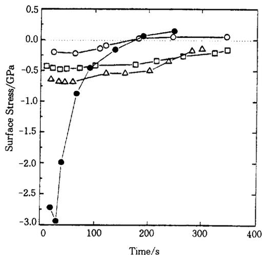
Fig. 6. Changes in surface stress with time during anodic oxidation of tungsten at an applied current density of  $0.08 \text{ mA cm}^{-2}$  in  $0.1 \text{ M H}_2\text{SO}_4$  solutions containing various concentrations of :  $\circ$ ,  $0 \text{ M NaCl}$ ;  $\square$ ,  $0.05 \text{ M NaCl}$ ;  $\triangle$ ,  $0.10 \text{ M NaCl}$ ;  $\bullet$ ,  $0.50 \text{ M NaCl}$ .
