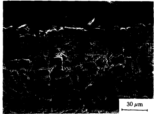
Fig. 8. Cross section of intergranular corrosion of Ti/C=6.2 steel with fast cooling rate heat cycle simulated at 1400°C and Huey tested.
