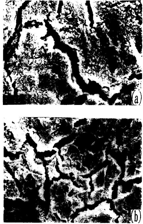
Fig. 5. Scanning electron micrograph showing corrosion morphology of (a) Mg-Li-Al and (b) Mg-Li-Al-Zr after potentiodynamic polarization test in a deaerated 0.03% NaCl buffered with KH_2PO_4 \cdot NaOH (PH7.00)
