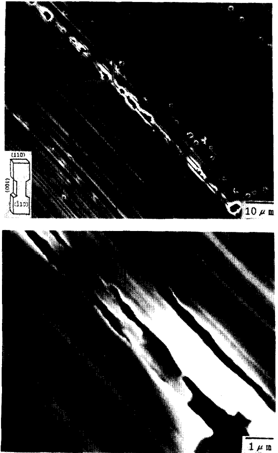
Fig. 2 Scanning electron micrographs of (110) surface corroded in cuprous ammoniacal solution in tension under slow strain rate ( 1.5 \times 10^{-5} /sec). (b) high magnification of (a)
