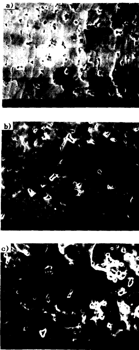
Fig. 11 Scanning electron micrographs of the corroded surface of aged ribbons at 200°C for 1hr
