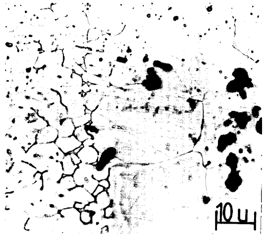
Fig. 15 Micro structure of CO 2 welded.
