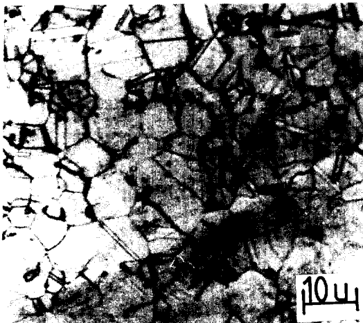
Fig. 8 Micro structure of 316 L.
