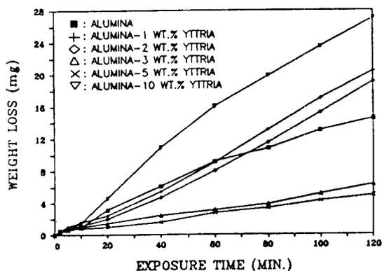
Fig. 6 Weight loss vs exposure time curves of plasma-sprayed alumina-yttria composite coatings.
