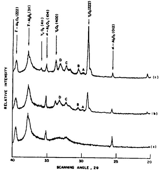
Fig. 2 X-ray diffraction of as-sprayed coatings: (a) alumina, (b) alumina-5 wt.% yttria, and (c) alumina-10 wt.% yttria.
