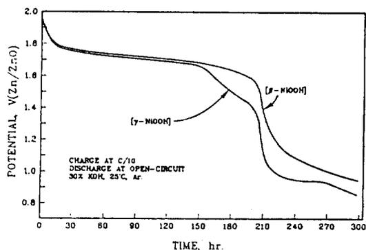
Fig. 7. Effect of crystalline phase of the nickel hydroxide electrode on the open-circuit potential behavior in 30% KOH at 25°C.
