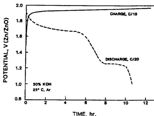
Fig. 3 Charge/discharge behavior as a function of time for the nickel hydroxide electrode in 30% KOH at 25°C.
