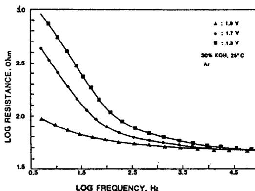
Fig. 4. Log frequency vs. log resistance of the nickel hydroxide electrode charged at different potential in 30% KOH at 25°C.
