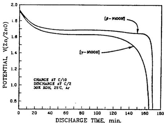
Fig. 6. Effect of crystalline phase of the nickel hydroxide electrode on the discharge behavior in 30% KOH at 25°C.
