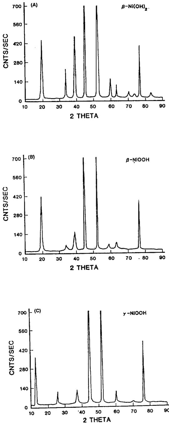
Fig. 1. X-ray diffraction patterns for : (A) as-impregnated,  $\beta\text{-Ni(OH)}_2$ , (B) after charge at C/10 for 12 hours,  $\beta\text{-NiOOH}$ , and (C) after overcharge at C/10 for 24 hours,  $\gamma\text{-NiOOH}$ .
