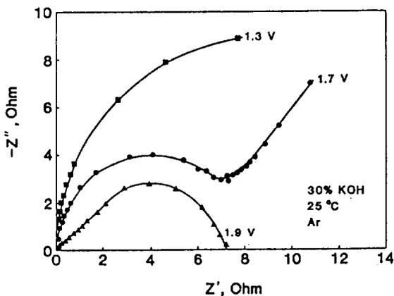
Fig. 5. Nyquist plot of the nickel hydroxide electrode at different potential in 30% KOH at 25°C.
