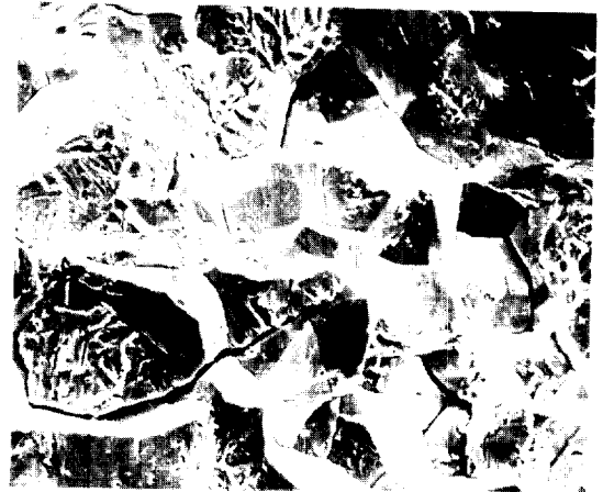
Fig. 10. Magnified view of intergranular fracture zone. (320 X).
