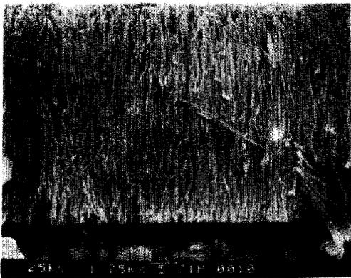
Fig. 6. Cross-section scanning electron micrograph of the Fe-1%Al-1%Hf alloy oxidized at 800°C for 121 hr showing the internal oxide morphology.
