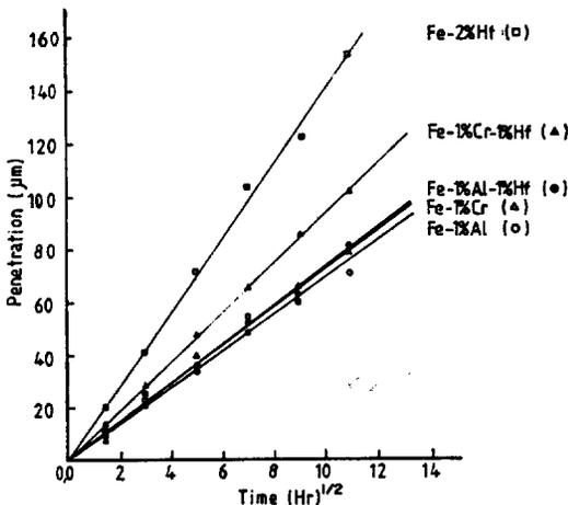
Fig. 1. Dependence of internal oxide growth rate on time of the five iron base alloys.
