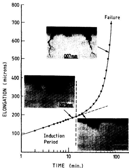
Fig. 3. Cross sectional metallographs of mill annealed E-Brite stressed 90% of the yield strength in boiling 42% LiCl+Thiourea at -460mV. Each metallograph was obtained from the specimen that was removed from the environment at the stage indicated by an arrow on the elongation-time curve.
