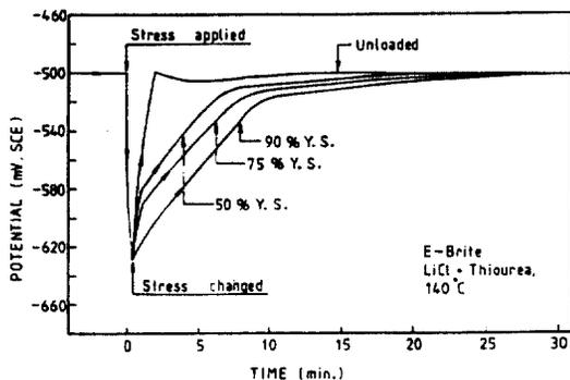
Fig. 6. Effect of stress change on repassivation revealed by corrosion potential-time curve for mill annealed E-Brite initially stressed to 90% of the yield strength in 42% LiCl+Thiourea at 140°C.
