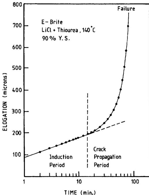
Fig. 2. Elongation as a function of time for mill annealed E-Brite stressed 90% of the yield strength and anodically polarized to  $-460\text{mV}$  in boiling 42% LiCl+Thiourea.
