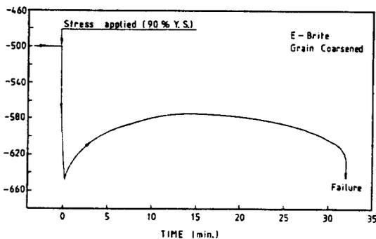
Fig. 8. Corrosion potential-time behavior of grain coarsened E-Brite upon loading of 90% of the yield strength in 42% LiCl+Thiourea at 140°C.
