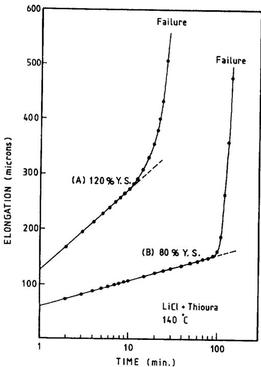
Fig. 5. Elongation-time curve for mill annealed E-Brite in boiling 42% LiCl+Thiourea, Showing effect of stresses on the crack initiation periods. (A) Loaded 120% of the yield strength. (B) Loaded 80% of the yield strength and anodically polarized to -460mV.
