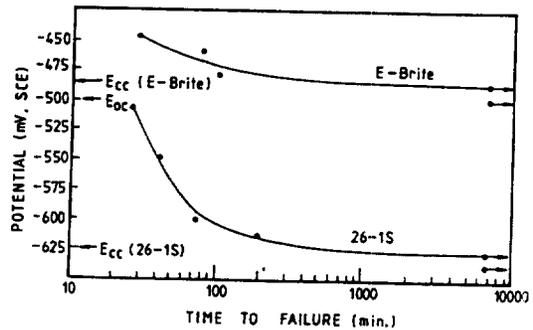
Fig. 1. Influence of applied potential on time failure of E-Brite and 26-1S respectively loaded 90% of the yield strength in 42% LiCl+Thiourea at 140°C.
