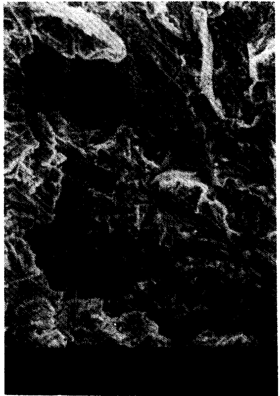
Fig. 14 SEM factograph of alloy No. H (0.291% N, 0.15% C) tested in 42% in MgCl 2 at an initial strain rate of 1.35 \times 10^{-5} \text{S}^{-1} .
