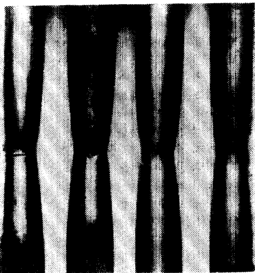
Fig. 11. Prestrained, heat treated (790°C/45min/oil, 370°C/60min/water), H-charged, and tensile tested 16)
