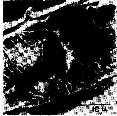
Fig. 4 Cracked surface of amorphous alloy(Fe 80 P 12 C 7 )
