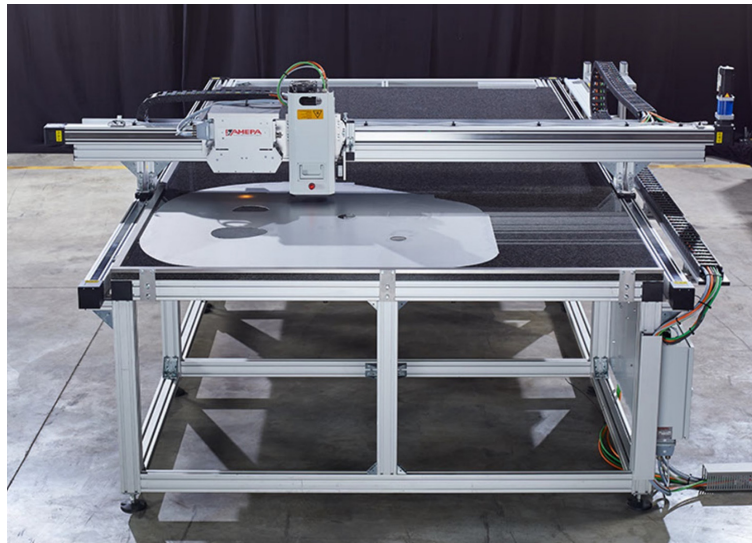
Fig. 8. With the Roughness Oilfilm Measurement (ROM) table, the oil film and roughness of individual plates of up to 2,000 × 4,000 mm size can be measured with high resolution
