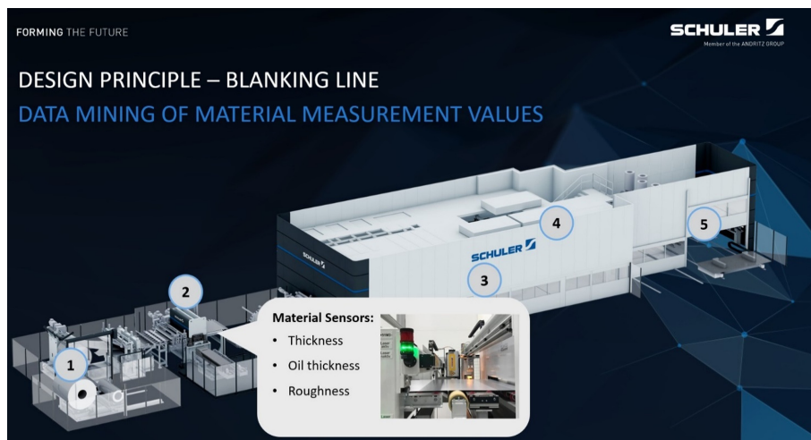
Fig. 3. The roughness and oil measuring systems are arranged after the leveller of the press line
