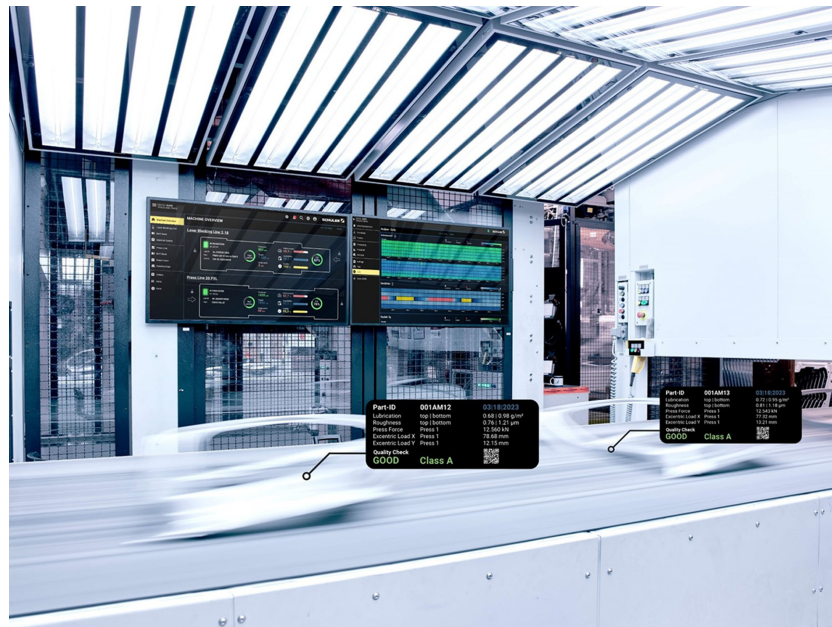
Fig. 10. The display at the inspection station shows the oil film and roughness values of each individual car body component
