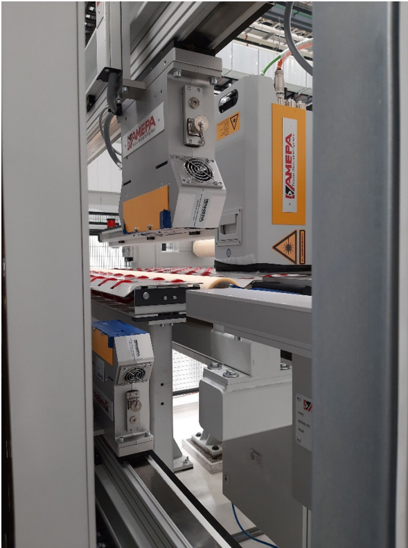
Fig. 5. Moving across the entire width of the strip, the sensors measure the oil film (left) and the surface roughness (right).
