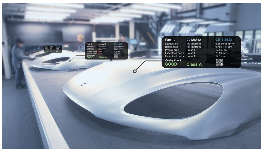
Fig. 2. Throughout the forming process, every bodyshell component is related to its specific measured data
