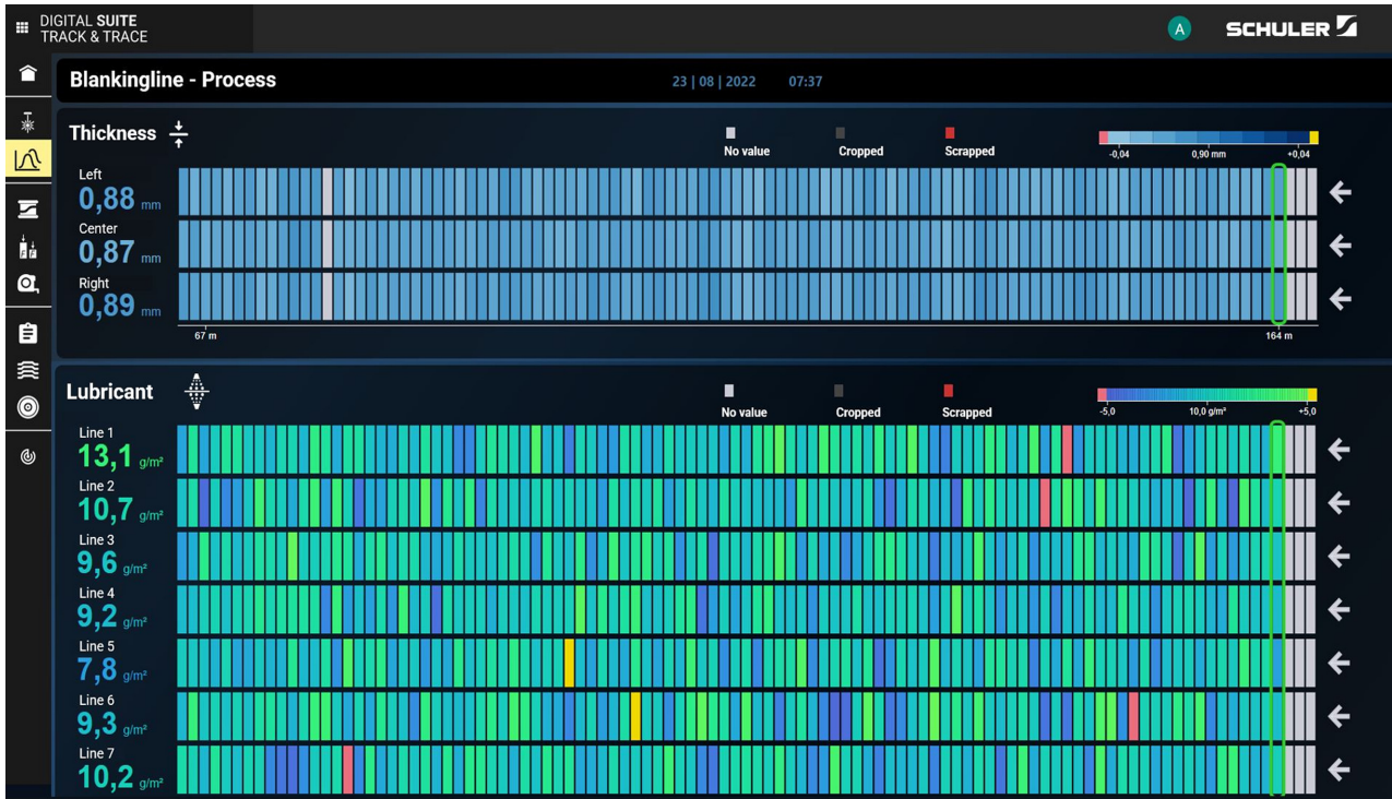
Fig. 6. The measured values are graphically displayed in a clearly structured form by meter of strip
