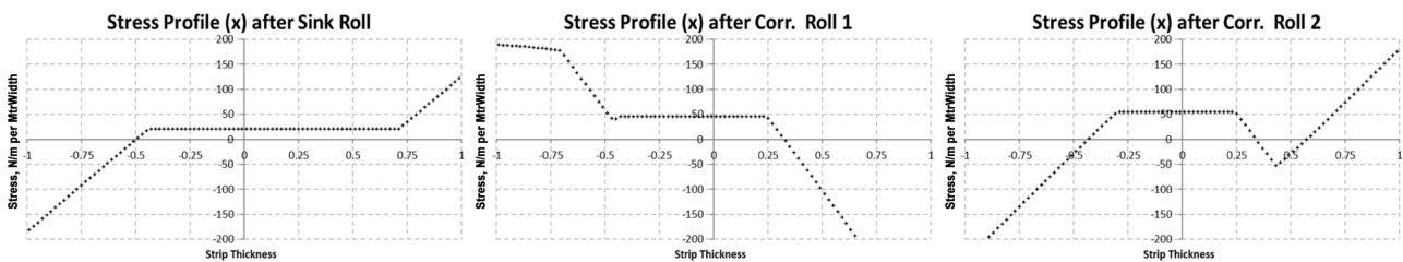
Fig. 11. Stress Profile in the length based direction (x) Intermesh = 29.85 mm
