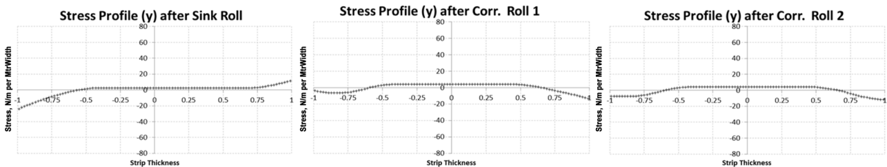
Fig. 10. Stress Profile in the transverse direction (y) Intermesh = 11.70 mm
