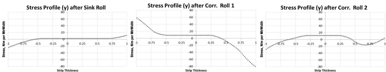
Fig. 12. Stress Profile in the transverse direction (y) Intermesh = 29.85 mm
