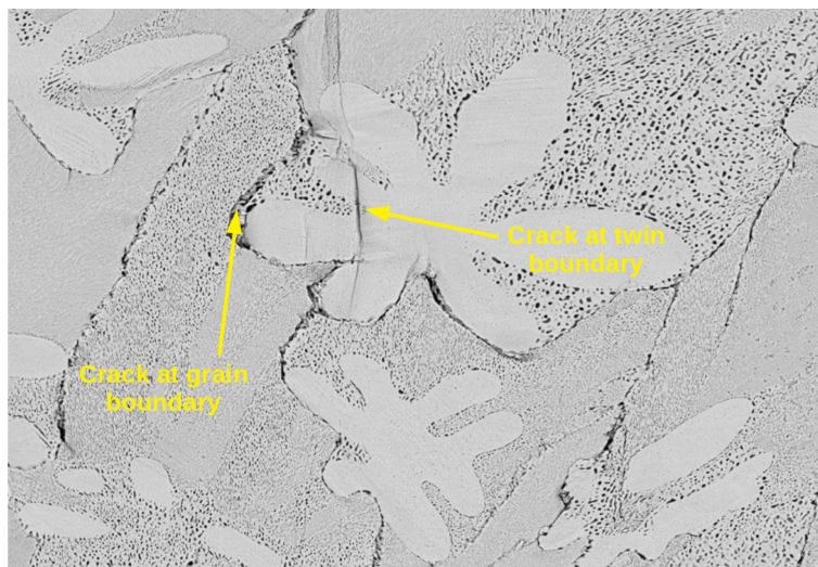
Fig. 12. SEM image of Zn-5Al coating after 15% of macroscopic strain showing a crack forming at twin boundaries
