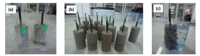
Fig. 2. Preparation of mortar specimens: (a) PVC molds after pouring the mortar, (b) mortar specimens after demolding, (c) curing of mortar specimens (14 days)
