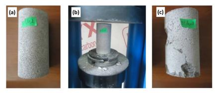
Fig. 4. Specimen conndition before and after compressive strength test : (a) Mortar specimen before compressive strength test, (b) specimen under compressive strength device, (c) specimen after compressive strength test
