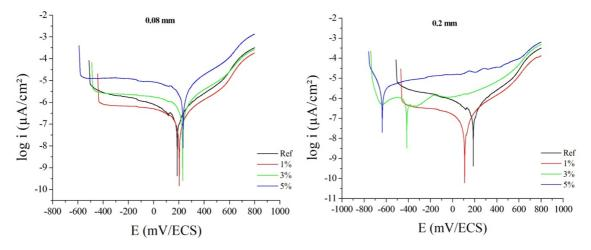
Fig. 7. Effect of cork concentration on the electrochemical behavior of steel
