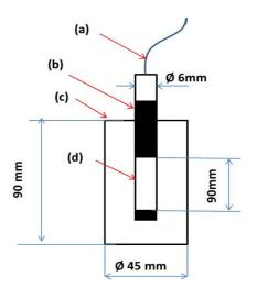
Fig. 1. Shape and size specimens: (a) electrical wire, (b) steel rebar, (c) mortar, (d) active surface of steel rebar
