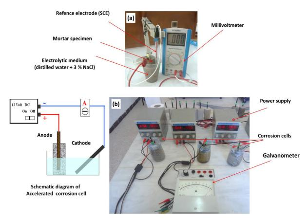
Fig. 3. Corrosion potential measurement and accelerated corrosion test
