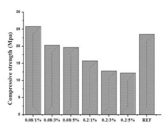
Fig. 10. Effect of granulometry and cork content on the compressive strength of the mortar
