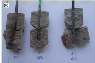
Fig. 9. Macrographs showing the steel surface condition after accelerated corrosion test: (a) granulometry = 0.08 mm, (b) granulometry = 0.2 mm
