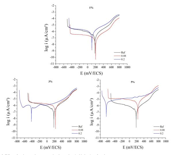
Fig. 8. Effect of cork granulometry on the electrochemical behavior of steel
