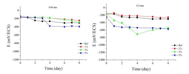
Fig. 5. Effect of cork content on the free potential evolution of steel
