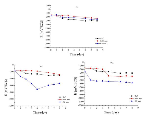
Fig. 6. Effect of cork granulometry on the corrosion potential evolution of steel
