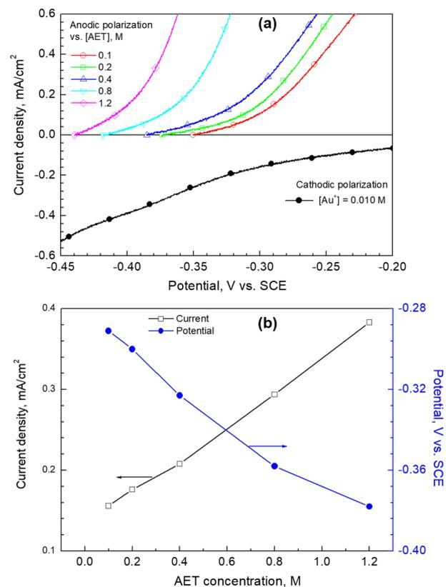
Fig. 4. Anodic polarization curve at different AET concentrations from 0.10 to 1.2 M (a), mixed potential interpreted from polarization curves and current density at the mixed potential (b), performed at 0.01 M Au<sup>+</sup>, 0.24 M TMA, pH 7.0 and temp. 80 °C
