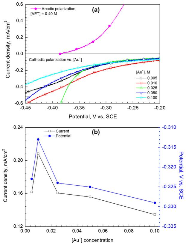
Fig. 5. Cathodic polarization curves at different Au<sup>+</sup> concentrations from 0.005 to 0.1 M (a), mixed potential interpreted from polarization curves and current density at the mixed potential (b), performed at 0.40 M AET, 0.24 M TMA, pH 7.0 and temp. 80 °C
