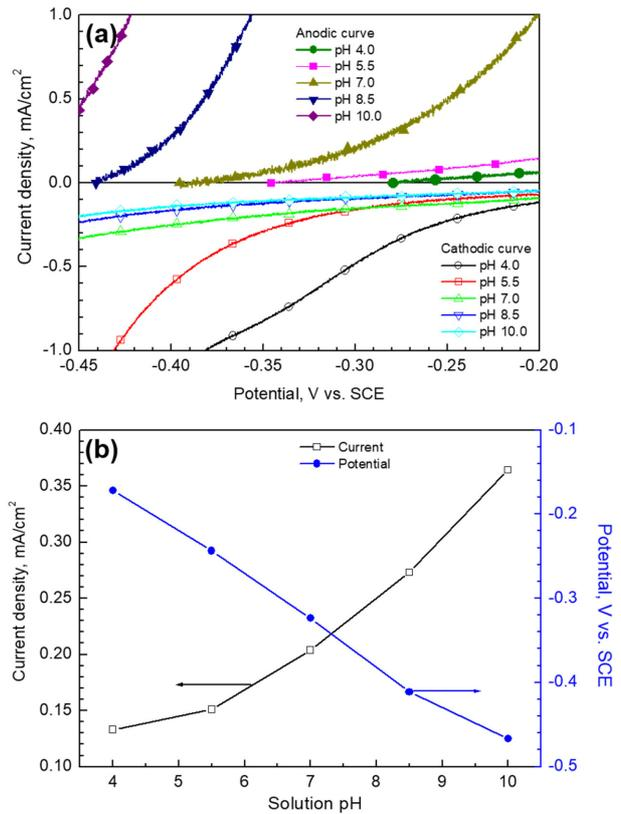
**Fig. 9.** Anodic and cathodic polarization curves at different solution pH (a), mixed potential interpreted from polarization curves and current density at the mixed potential (b), performed at 0.01 M Au<sup>+</sup>, 0.40 M AET, 0.24 M TMA, and temp. 80 °C
