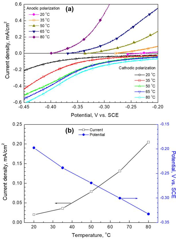
**Fig. 8.** Anodic and cathodic polarization curves at different temperatures (a), mixed potential interpreted from polarization curves and current density at the mixed potential (b), performed at 0.01 M Au<sup>+</sup>, 0.40 M AET, 0.24 M TMA, and pH 7.0
