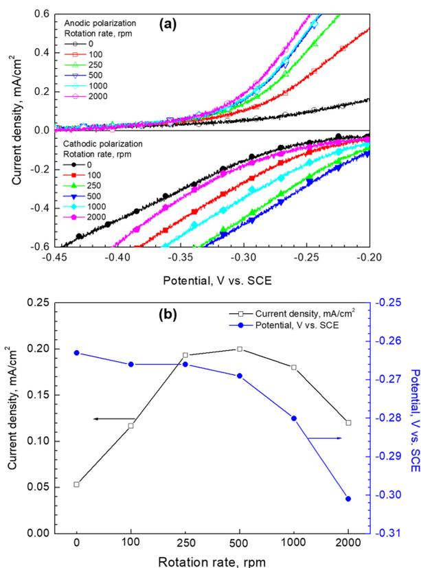
Fig. 3. Anodic and cathodic polarization curves of the basic electroless gold solution at different electrode rotation rates from 0 to 2000 rpm (a), mixed potential interpreted from polarization curves and current density at the mixed potential (b)
