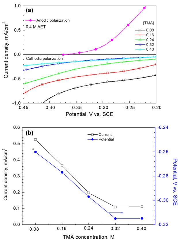
Fig. 7. Cathodic polarization curve at different TMA concentrations from 0.08 to 0.40 M (a), mixed potential interpreted from polarization curves and current density at the mixed potential (b), performed at 0.01 M  $\text{Au}^3$ , 0.40 M AET, pH 7.0 and temp. 80 °C
