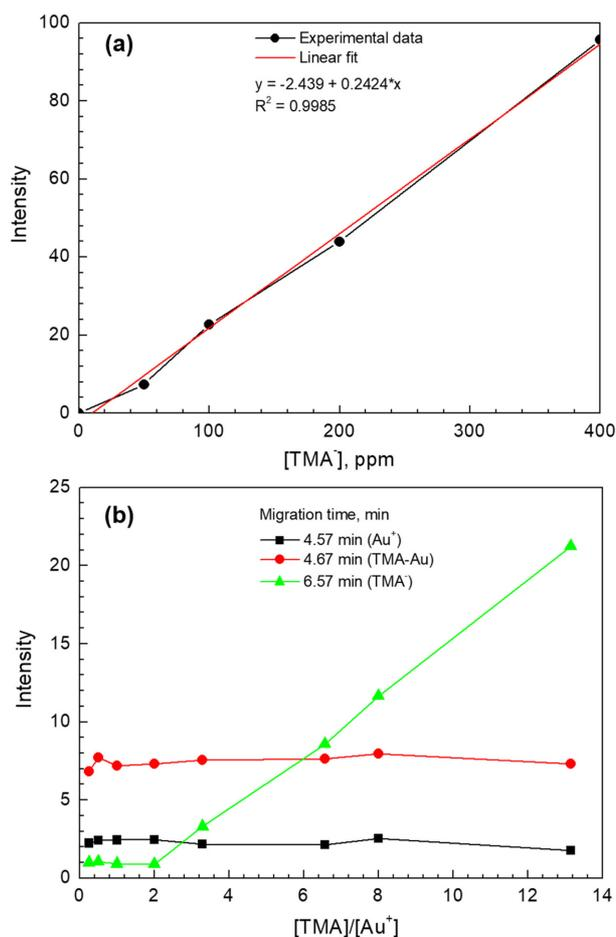
Fig. 1. CE calibration curve of the basic TMA solution (a) and CE peak intensities of  $\text{Au}^+$ , TMA-Au, and TMA at different [TMA]/[Au<sup>+</sup>] concentration ratios. The migration time of  $\text{Au}^+$ , TMA-Au, and TMA was 4.57, 4.67, and 6.57 min, respectively
