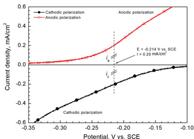
Fig. 2. Anodic and cathodic polarization curves of the basic electroless gold plating solution (Table 2)
