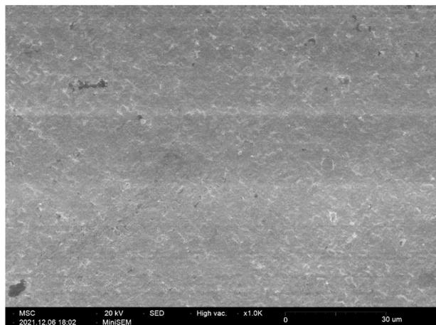
**Fig. 10.** SEM morphology of electroless gold plated on electroless nickel-phosphorus film, obtained from the basic electroless gold solution with a plating time of 30 min
