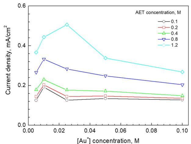
Fig. 6. Current density at the mixed potential interpreted from the polarization curve at different Au<sup>+</sup> and AET concentrations. Polarization curves performed at 0.24 M TMA, pH 7.0, temp. 80 °C and electrode rotation rate of 500 rpm
