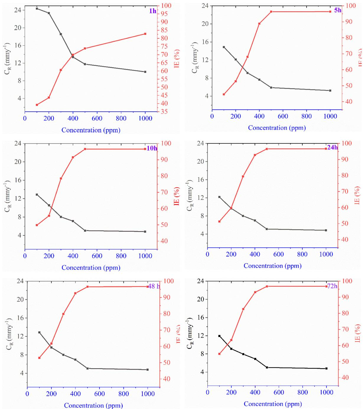
**Fig. 2.** The rate of corrosion rate and inhibition efficiency of the tested inhibitor at different concentrations (100-1000 ppm) for mild steel versus the immersion time (1-72 h), at 303 K
