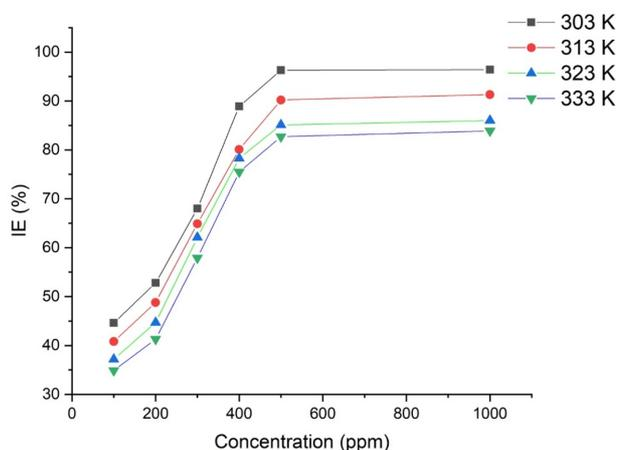
**Fig. 3. The inhibition efficiency of the tested inhibitor at different concentrations (100-1000 ppm) for mild steel versus the Temperature (303-333 k), for 5 h as immersion time**
