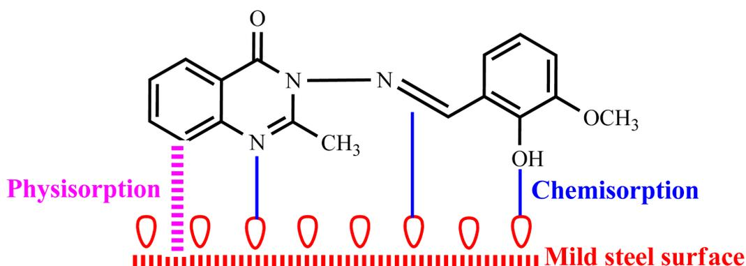
**Fig. 7. Postulated inhibition mechanism of SB-Q on mild steel surface in corrosive medium**
