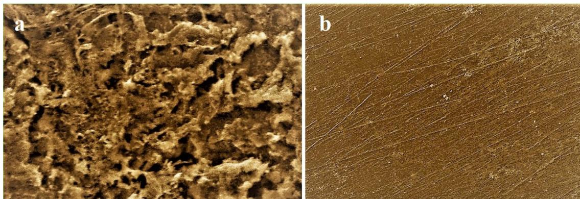
Fig. 5. SEM images of mild steel coupon surfaces: (a) after 10 h exposure in 1.0 M HCl environment without addition of SB-Q, and (b) after 10 h exposure in 1.0 M HCl environment with addition of 500 ppm of SB-Q
