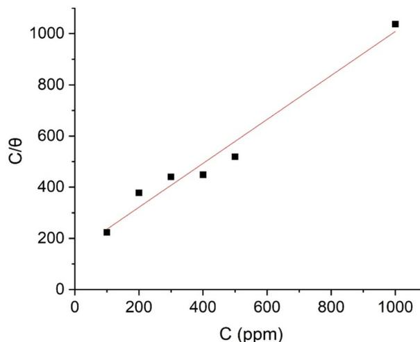
Fig. 4. Langmuir adsorption isotherm plot for various concentration at 303 K
