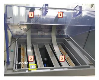
Fig. 7. It is to check the correlation between the position of the anode attached to the specimen and the corrosive environment in the exposure chamber. The specimen on the left in the figure is when the anode of dc module installed on the bottom of the exposure chamber, and the specimen on the right is no treatment. Two scratches – Site1, Site2 - were created on the specimen
