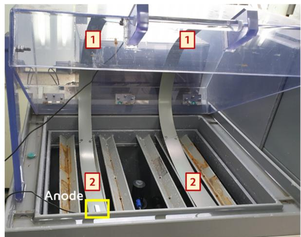
Fig. 7. It is to check the correlation between the position of the anode attached to the specimen and the corrosive environment in the exposure chamber. The specimen on the left in the figure is when the anode of dc module installed on the bottom of the exposure chamber, and the specimen on the right is no treatment. Two scratches – Site1, Site2 - were created on the specimen
