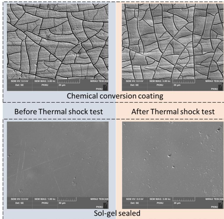
Fig. 3. The SEM image of chemical conversion coating and sol-gel sealed specimens with thermal shock test
