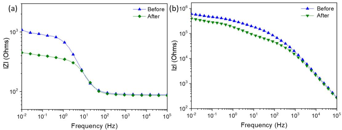
Fig. 4. Bode plots of (a) chemical conversion coating and (b) Sol-gel sealed specimens before and after thermal shock test
