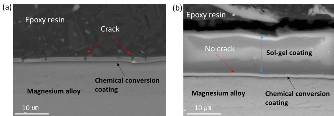
**Fig. 7. The cross-section of SEM images of specimens. (a) chemical conversion coating and (b) sol-gel sealed specimen**
