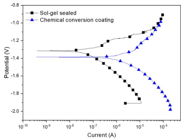
Fig. 6. The results of the potentiodynamic polarization test of specimens
