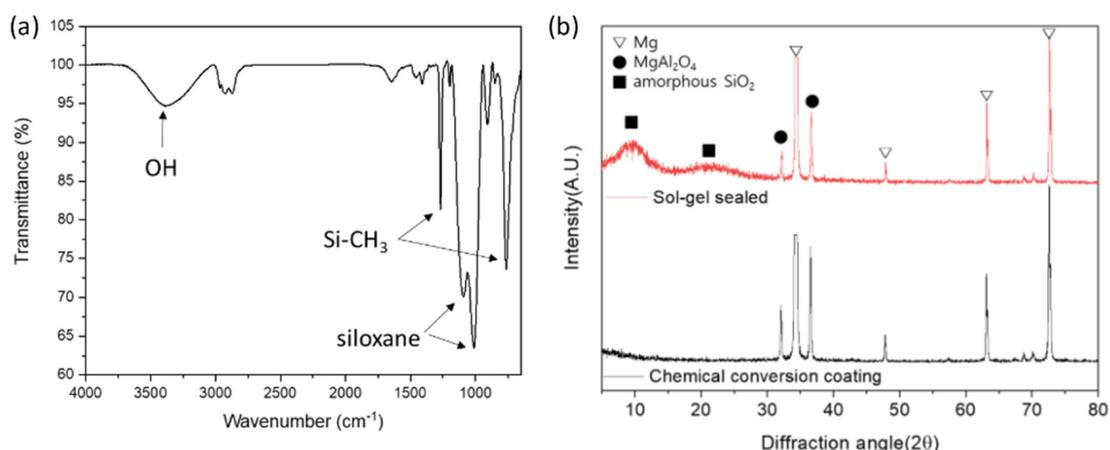
Fig. 2. (a) FT-IR spectrum of sol-gel sealed coating surface and (b) XRD spectra of sol-gel sealed coating and chemical conversion coating
