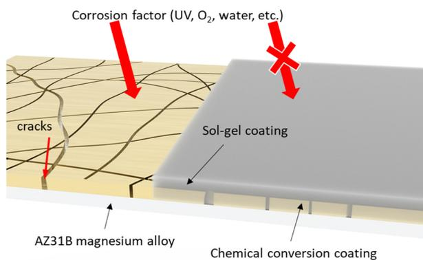
**Fig. 1. The schematic illustration of dual chemical conversion and sol-gel coating on AZ31B magnesium alloy**
