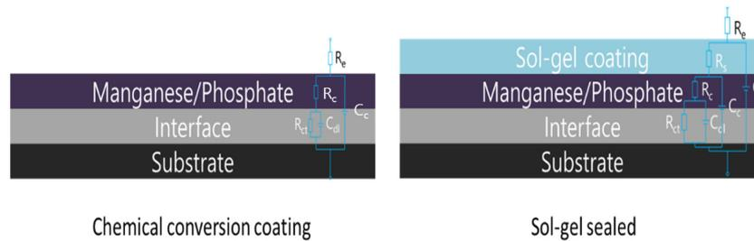
Fig. 5. The schematic illustration of electrical circuit components of each coating specimens
