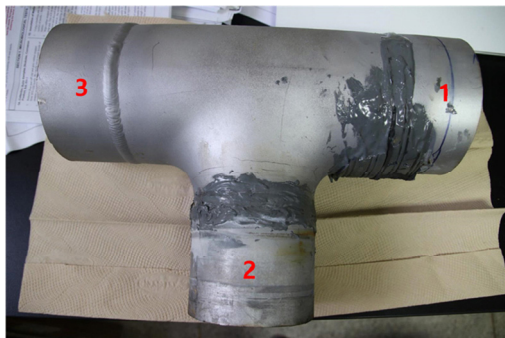
Fig. 2 A OM image representing a damaged T-type connector.
