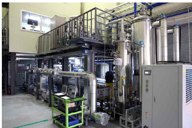
Fig. 1 Flow Accelerated Corrosion Testing System (FACTS).
