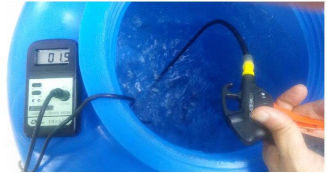
Fig. 3 Nitrogen bubbling to reduce the dissolved oxygen concentration in the water tank.
