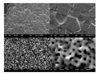
Fig. 8 Surface morphology for titanium substrate after being anodized in  $H_2SO_4$  solution for 15 minutes.
