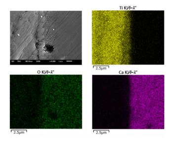
Fig. 9 Cross section profile by SEM and elements distribution by EDS for plasma sprayed Zn doped HAp coating with an intermediate layer prepared by titanium anodizing in  $H_2SO_4$  solution for 15 min.
