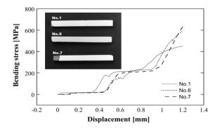
Fig. 5 Results of three-point bending test for plasma sprayed Zn doped HAp coatings under different conditions (shown in Table 1 and Table 2).
