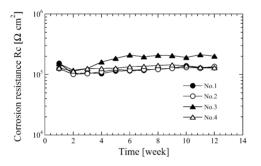
Fig. 2 Changes in corrosion resistance  $R_C$  for Zn doped HAp plasma sprayed coatings with Ti plasma sprayed intermediate layer in Hanks' solution at 37 °C. samples were prepared under conditions shown in Table 1.
