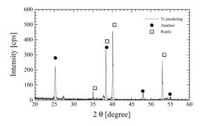
Fig. 7 X-ray diffraction result for the surface of titanium substrate after being anodized in  $H_2SO_4$  solution for 15 minutes.
