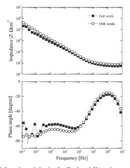
Fig. 1 Impedance behavior for Zn doped HAp plasma sprayed coating with Ti plasma sprayed intermediate layer after 2 weeks immersion in Hanks' solution at 37 °C. samples were prepared under conditions shown in Table 1.
