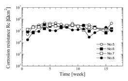
Fig. 4 Changes in corrosion resistance in Hanks' solution at 37 °C  $R_C$  for Zn doped HAp plasma sprayed coatings with an intermediate layer prepared by titanium anodization. The samples were prepared under the conditions shown in Table 2.
