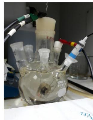
Fig. 2 EPR corrosion experiment cell.
