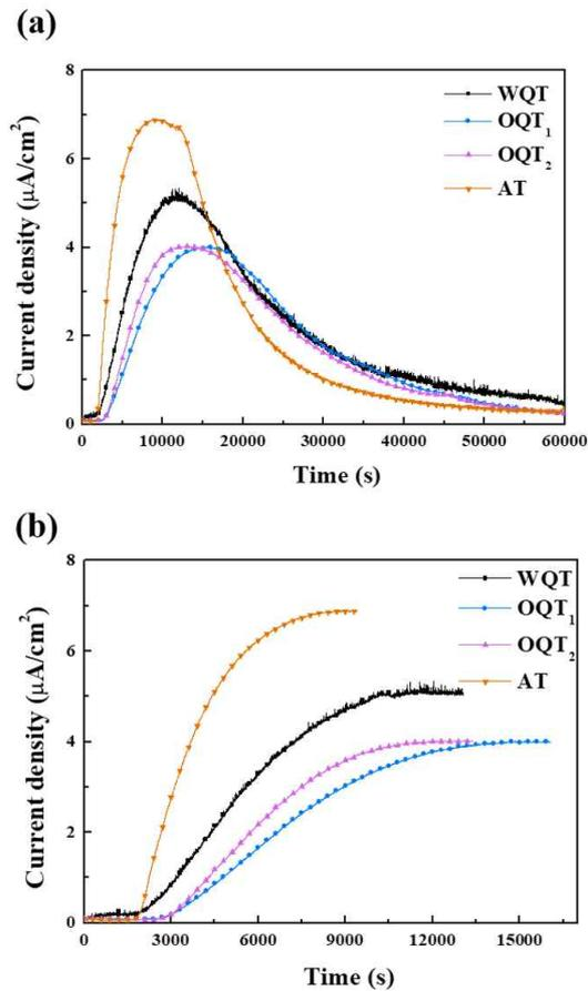
Fig. 6 (a) H permeation curves of the four tested samples, and (b) their rising permeation transients.
