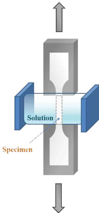
Fig. 2 Schematic diagram of the SSRT apparatus.
