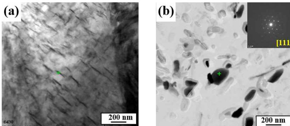
Fig. 4 TEM observation: (a) fine needle shaped  $\epsilon$ -Fe<sub>2.4</sub>C in the WQT sample and (b) coarse spherical shaped Fe<sub>3</sub>C in the AT sample.
