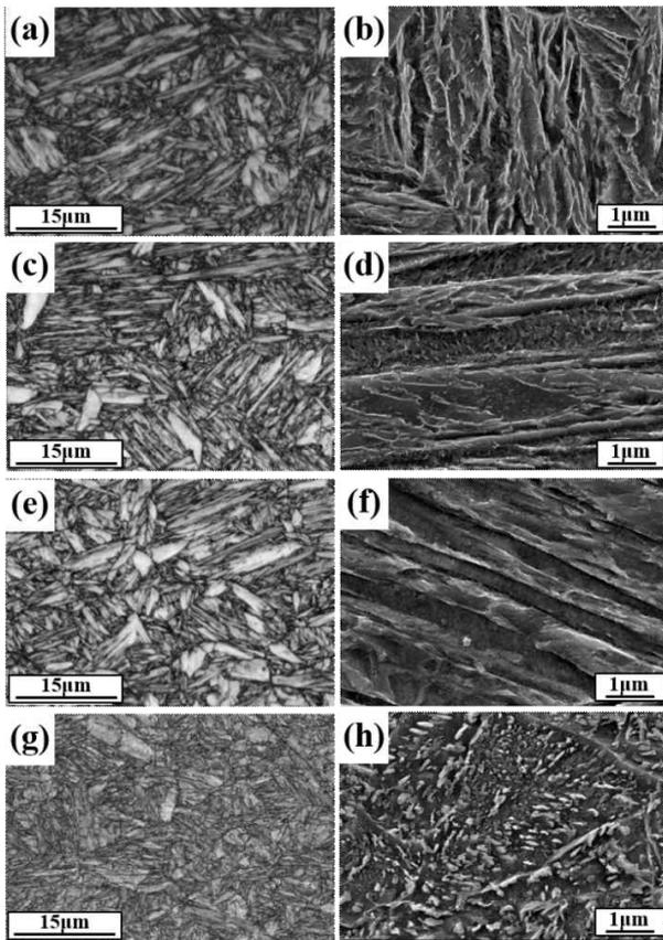
Fig. 3 Microstructure observed by EBSD (a, c, e, g) and FE-SEM (b, d, f, h): (a-b) WQT, (c-d) OQT<sub>1</sub>, (e-f) OQT<sub>2</sub>, and (g-h) AT samples.
