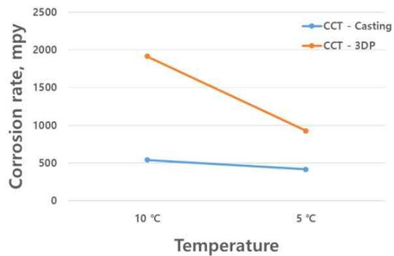
Fig. 7 CPT, CCT determination by corrosion rate for 316L.
