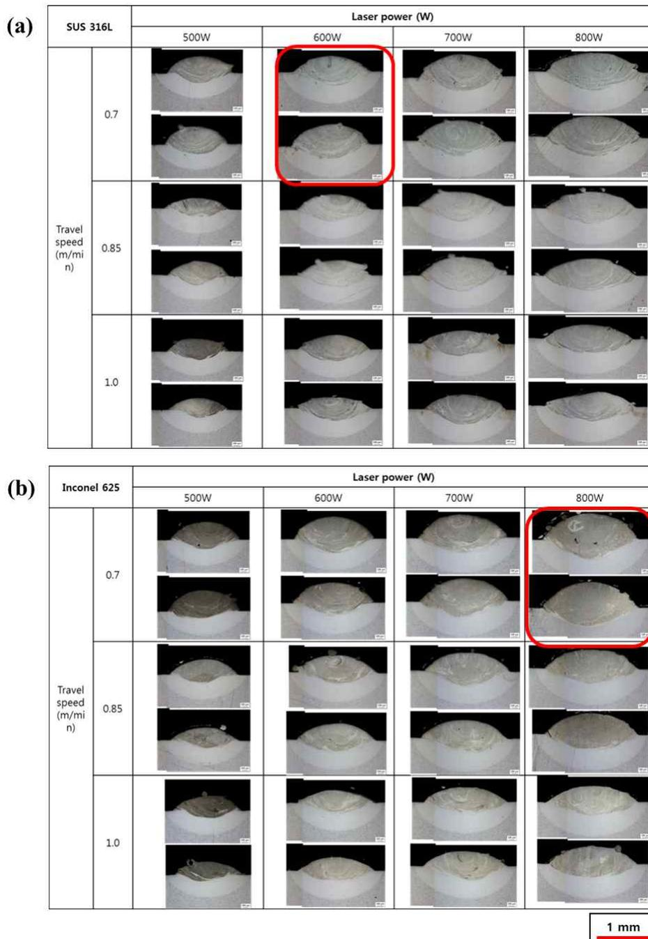
Fig. 4 Dimensions of the deposited layers with various conditions, (a) 316L, (b) alloy 625, optimized conditions are highlighted in red square.
