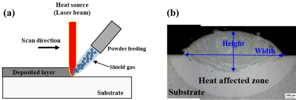
Fig. 2 Schematic of DED process (a), deposited layer by DED (b) [6].
