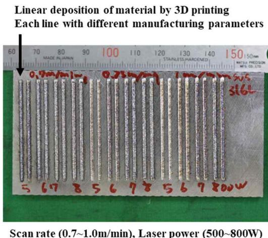
Fig. 3 Deposited lines with the different process conditions.
