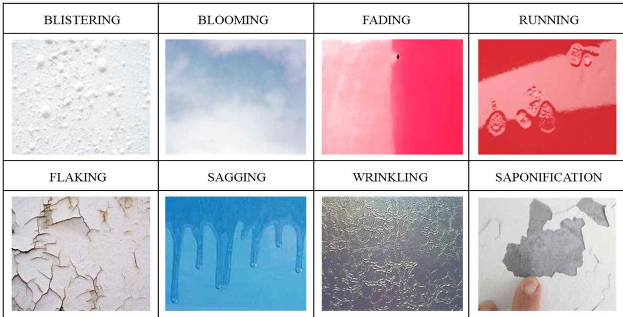
Fig. 3 Common Defects in Paint Works.
