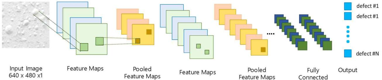
**Fig. 2 Convolutional Neural Network for Painting Surface Inspection.**
