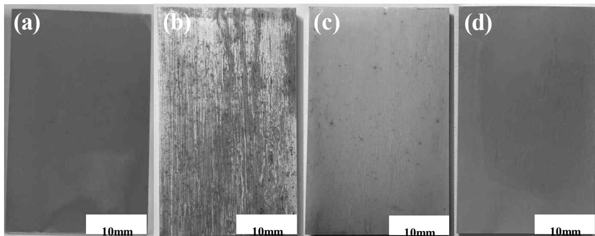
**Fig. 5** Surface observation on AZ31B Mg alloy by digital camera after immersion test for 96 hr; (a) 0.01 M NaOH, (b) 0.01 M NaOH + 0.01 M NaCl, (c) 0.01 M NaOH + 0.01 M NaCl + 0.5 M SB, (d) 0.01 M NaOH + 0.01 M NaCl + 0.5 M SB + 0.005 M SDBS.
