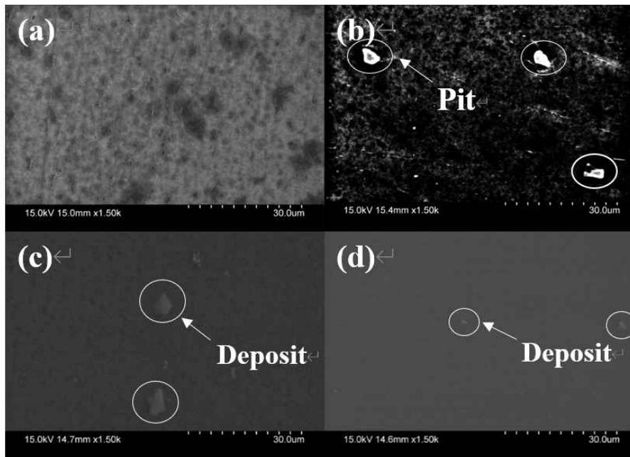
**Fig. 7** Surface microscopy of AZ31B Mg alloy by SEM after immersion test for 96 hr; (a) 0.01 M NaOH, (b) 0.01 M NaOH + 0.01 M NaCl, (c) 0.01 M NaOH + 0.01 M NaCl + 0.5 M SB, (d) 0.01 M NaOH + 0.01 M NaCl + 0.5 M SB + 0.005 M SDBS.
