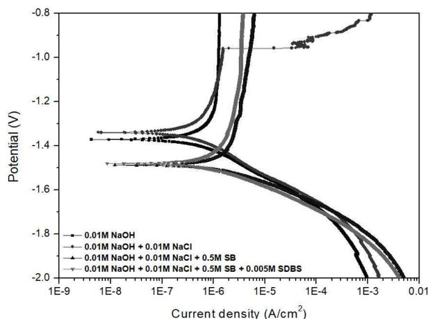
**Fig. 4** Potentiodynamic polarization curves of AZ31B Mg alloy for the 0.01 M NaOH with different NaCl concentration in aerated condition in addition with 0.5 M SB and/or 0.005 M SDBS at the scan rate of 0.175 mV/s.
