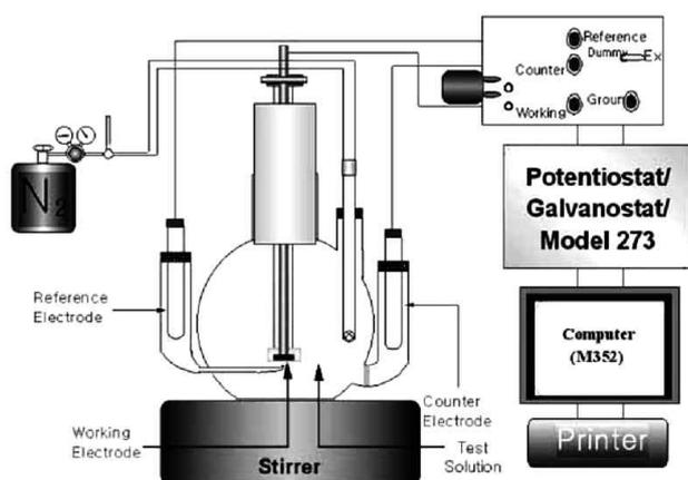
Fig. 1 The experimental set-up for electrochemical test.
