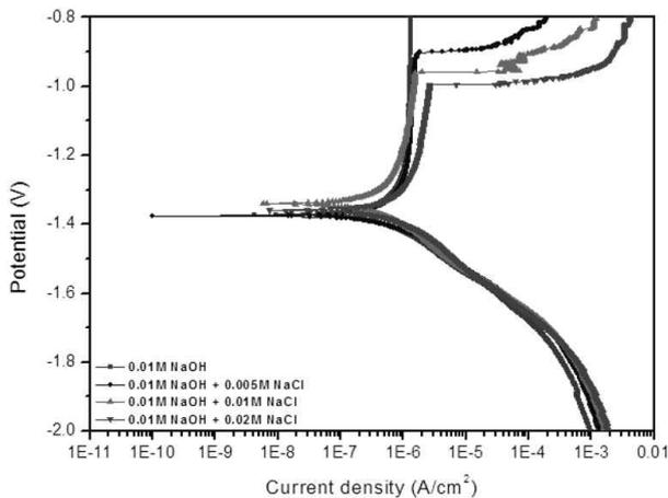
**Fig. 3** Potentiodynamic polarization curves of AZ31B Mg alloy for the 0.01 M NaOH with different NaCl concentration in aerated condition at the scan rate of 0.175 mV/s.
