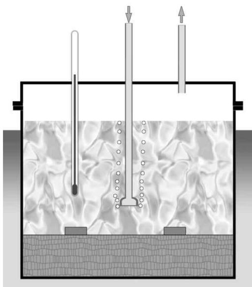
Fig. 2 Schematic drawing of immersion test.
