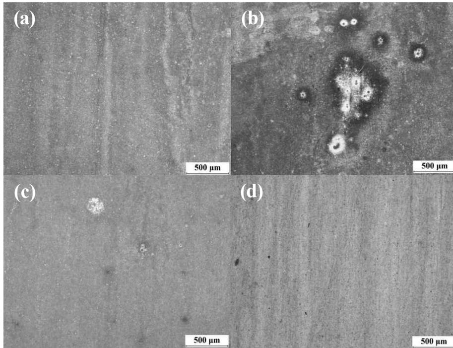
**Fig. 6** Surface microscopy of AZ31B Mg alloy by optical microscopy after immersion test for 96 hr; (a) 0.01 M NaOH, (b) 0.01 M NaOH + 0.01 M NaCl, (c) 0.01 M NaOH + 0.01 M NaCl + 0.5 M SB, (d) 0.01 M NaOH + 0.01 M NaCl + 0.5 M SB + 0.005 M SDBS.
