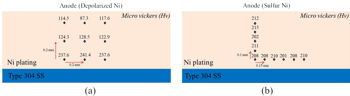
Fig. 6 Micro Vickers hardness on nickel plating (a) with depolarized Ni anode, (b)with Sulfur Ni anode.
