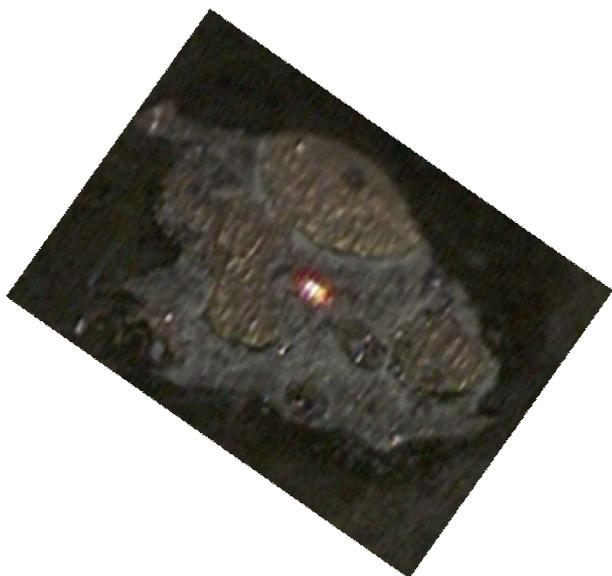
Fig. 2 Alignment of the specimen for the micro-XRD measurement with the help of a laser beam; the bright spot at the center shows the laser beam on the corrosion pit found in the region 3 (see Fig. 5).
