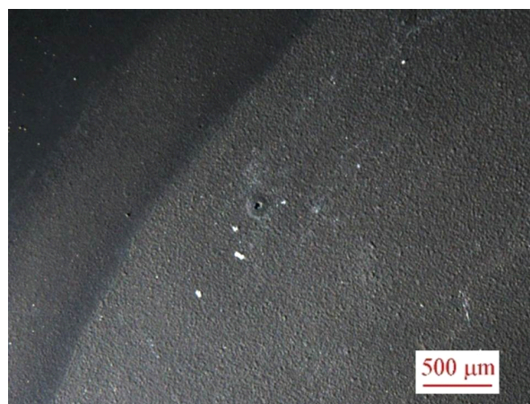
Fig. 14 surface of sample 1S after 10 hours of contact with commercial remover.
