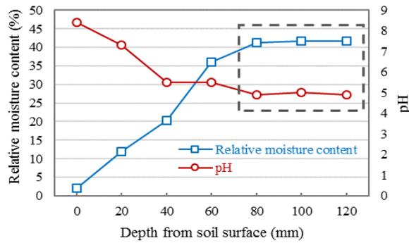
**Fig. 3** Relative moisture content and pH with depth from the soil surface.
