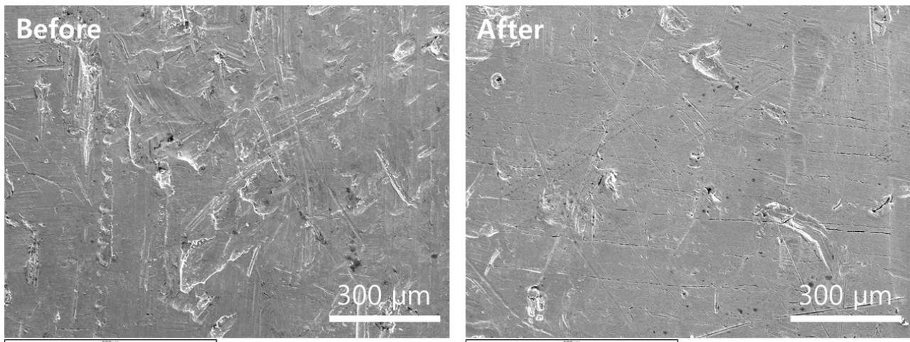
Fig. 6 SEM images of copper layer before and after the immersion corrosion test.
