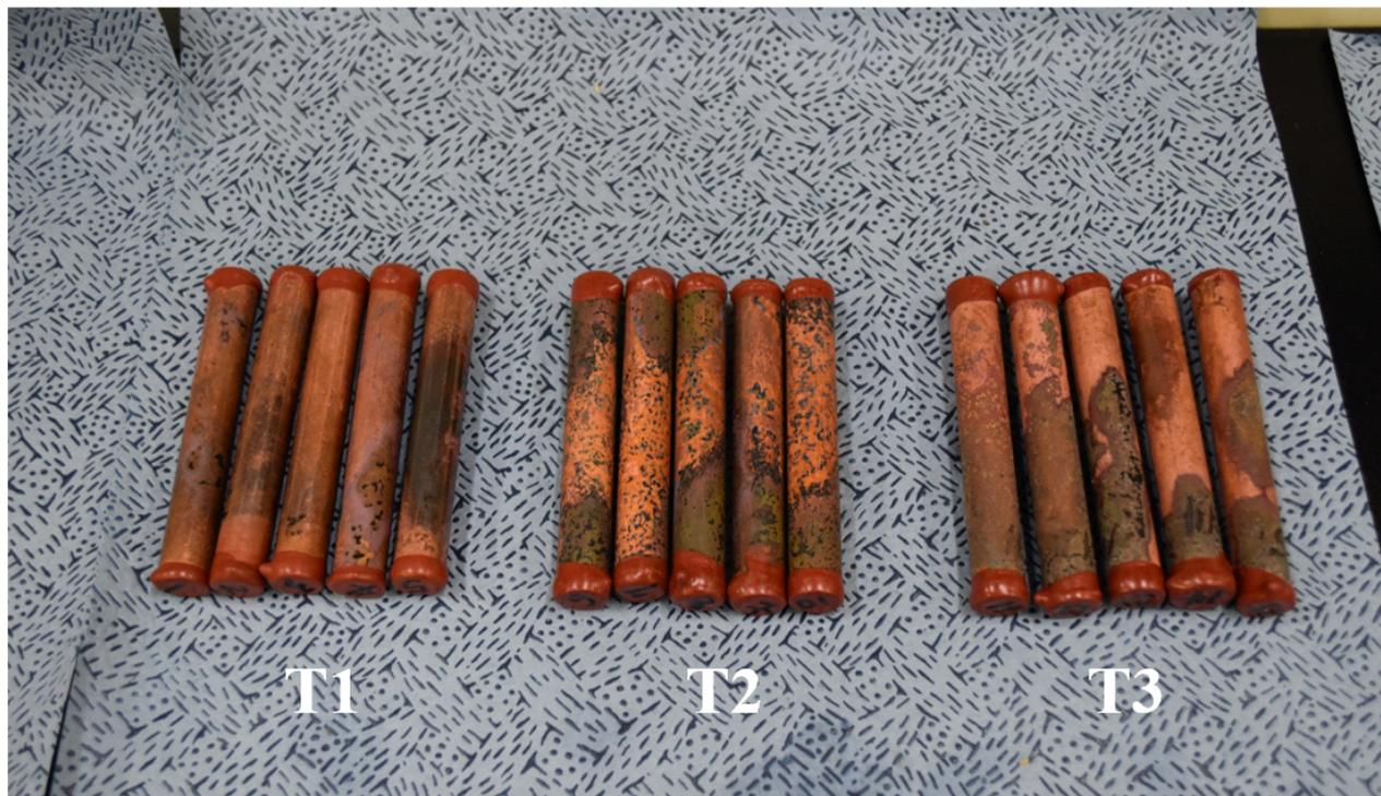
Fig. 7 Specimens after one month of the improved accelerated corrosion test.
