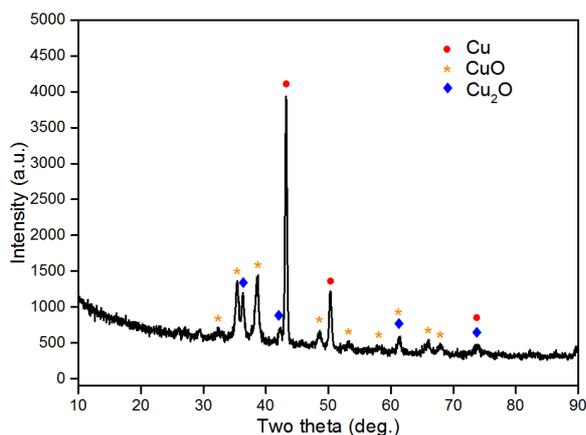
Fig. 5 X-ray diffraction pattern of the aged copper bonded grounding material.
