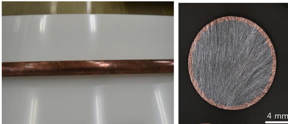
Fig. 4 Naturally degraded copper bonded grounding material after cleaning and cross-section image.
