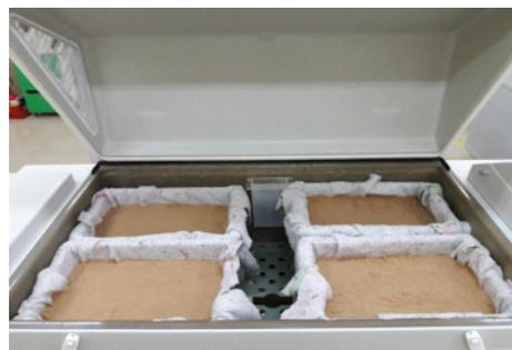
**Fig. 2 Inside of improved cycle corrosion tester with the soil baskets.**
