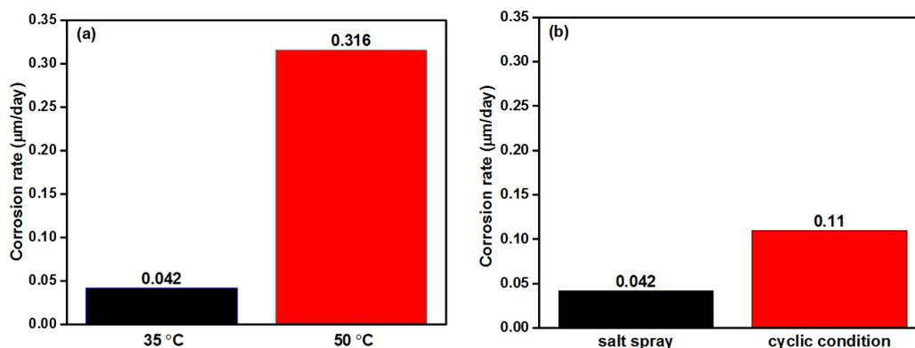
**Fig. 8 Comparison of the corrosion rates by (a) temperature (35 °C and 50 °C) and (b) spray conditions (continuous salt spray and salt spray-dry-wet cycle).**
