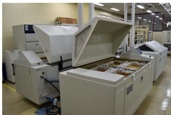
**Fig. 1 Cycle corrosion testers.**
