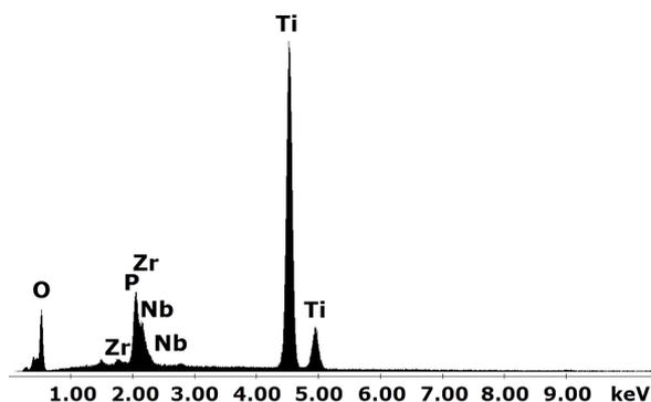
Fig. 3 EDS spectrum of oxide nanolayer on Ti-15Zr-5Nb alloy surface.
