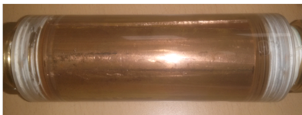
Fig. 5 A closed model system made of an acryl tube and brass fittings for performing experiment of hydrazine reaction and corrosion inhibition. Notice the brightness of the tube surface and edge even after 10 months of experiment.
