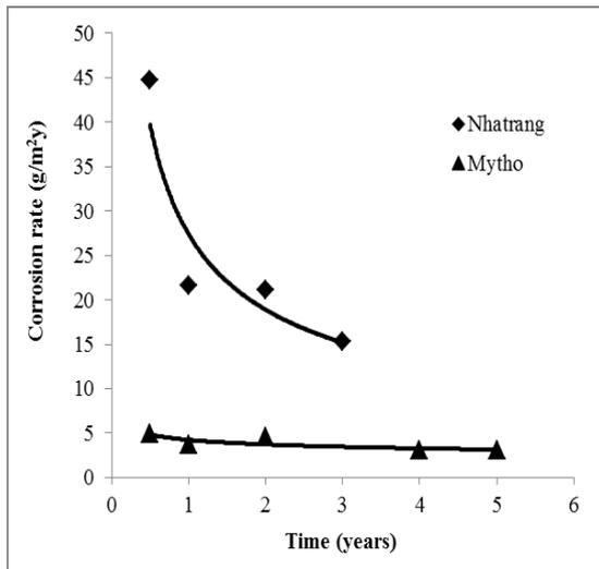
Fig. 1 Time dependence of corrosion rate for zinc coatings.
