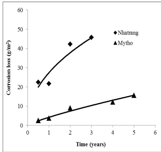
Fig. 2 Time dependence of mass loss for zinc coatings.
