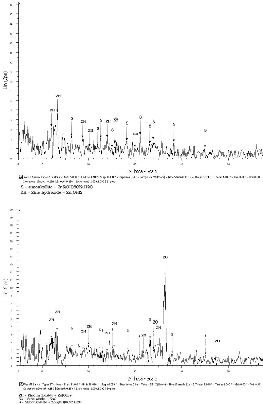
Fig. 5 XRD diagram of the samples after five years of exposure testing. (upper: Nhatrang; lower: Mytho)
