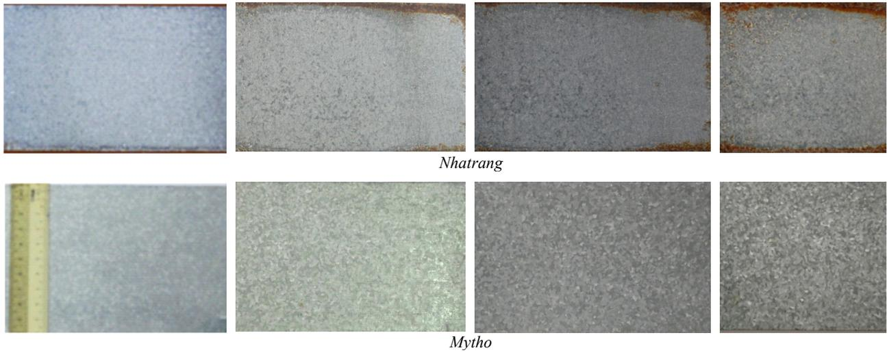
**Fig. 3 Surface appearance of the tested samples after first, third, fourth and fifth year of exposure.**
