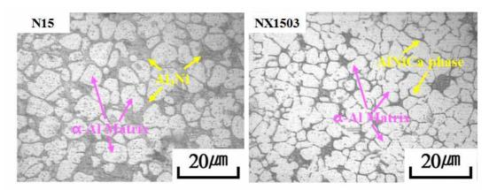
Fig. 2 Microstructures of high pressure die cast N15 and NX1503 Al alloys.
