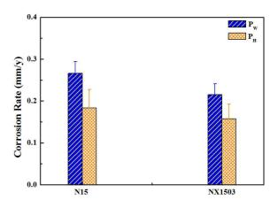
Fig. 8 Comparison of corrosion rates ( $P_{\rm W}$  and  $P_{\rm H}$ ) of N15 and NX1503 Al alloys after 72 h of immersion in 3.5% NaCl solution.
