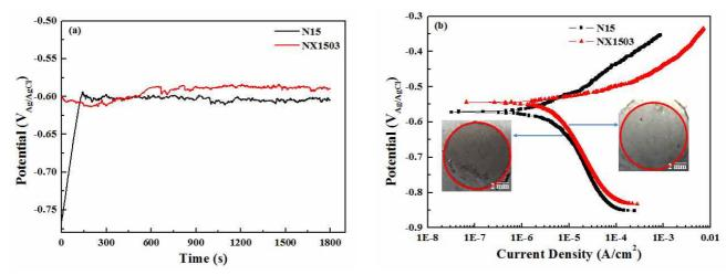
Fig. 3 (a) OCP and (b) Potentiodynamic polarization curves of N15 and NX1503 Al alloys in 3.5% NaCl solution.
