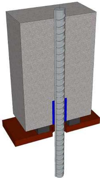
Fig. 2 Schematic drawing of the standard pull-out test.
