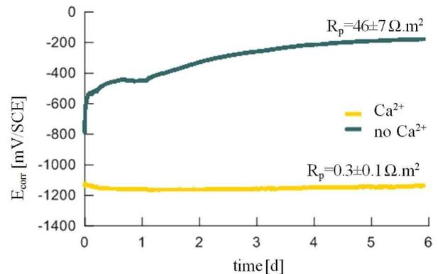
Fig. 4  $E_{corr}$  in dependence on time for zinc in a solution of pH 12.6 containing or not containing calcium ions.
