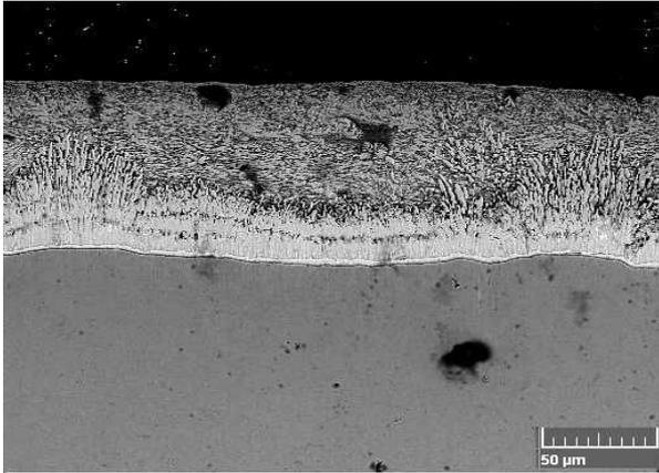
Fig. 1 Structure of the coating at the hot-dip galvanized steel specimen.
