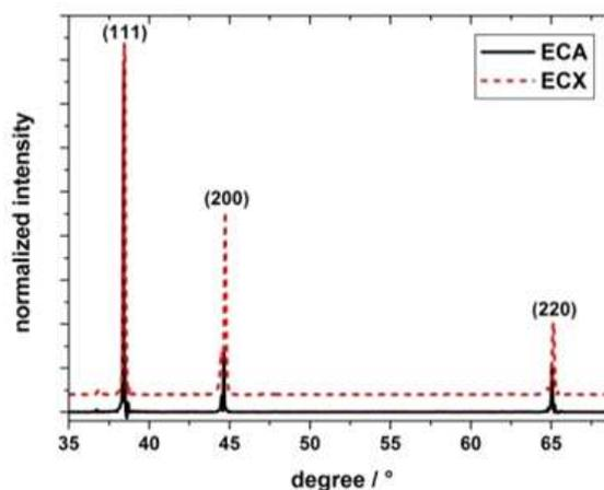
**Fig. 2.** XRD spectra of electrodeposited 20 µm thick Al coatings made by ECA and ECX (dotted line) process.
