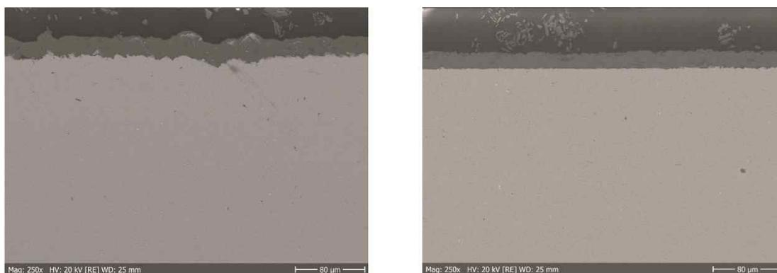
**Fig. 3.** Cross sections of electroplated Al layers (20 μm) on Eurofer: ECA process - 10 mA/cm<sup>2</sup> t = 2h (left) and ECX process - 20 mA/cm<sup>2</sup>, t = 1h (right).
