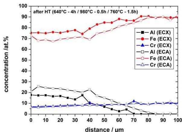
Fig. 5. EDS line scan of Eurofer, coated with 20  $\mu\text{m}$  thick Al by ECA and ECX (filled-out symbols) after heat treatment.
