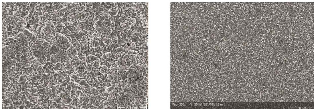
**Fig. 1.** SEM images of surfaces of electroplated Al layer (20 µm thick) on Eurofer steel: ECA process - 10 mA/cm<sup>2</sup> (left) and ECX process - 20 mA/cm<sup>2</sup> (right).
