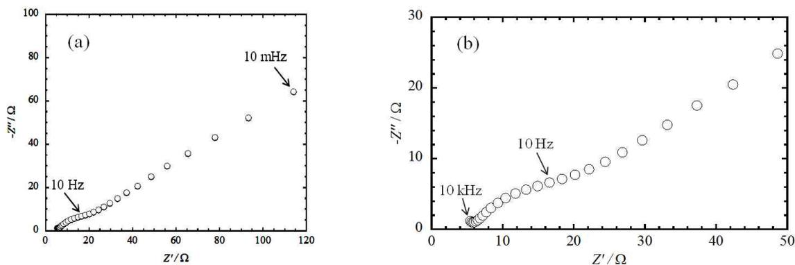
Fig. 3. Impedance spectrum of the Cu in  $0.5$  M NaCl containing  $5$  mM NaHCO<sub>3</sub> (a) Full range, (b) Expanded of the high frequency range.
