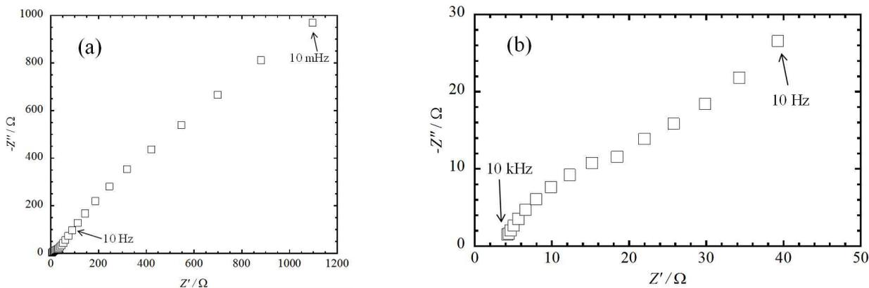
**Fig. 4.** Impedance spectrum of the Cu-Zn alloy in 0.5M NaCl containing 5 mM NaHCO<sub>3</sub>(a) Full range, (b) Expanded of the high frequency range.
