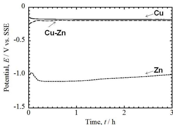
Fig. 1. Changes of the rest potential  $E_{\text{rest}}$  of Cu, Zn, and the Cu-Zn alloy during the immersion test.
