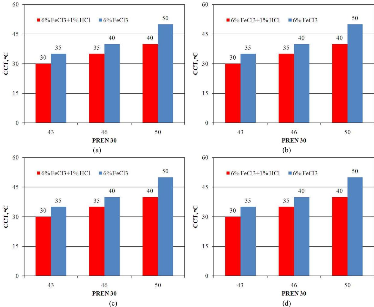
**Fig. 10.** CCT of the duplex stainless steel determined in 6 % FeCl<sub>3</sub> + 1 % HCl and 6 % FeCl<sub>3</sub> solution; (a) plate, and (b) round bar (D; 35 mm), (c) round bar (D; 25 mm), (d) round bar (D; 15 mm).
