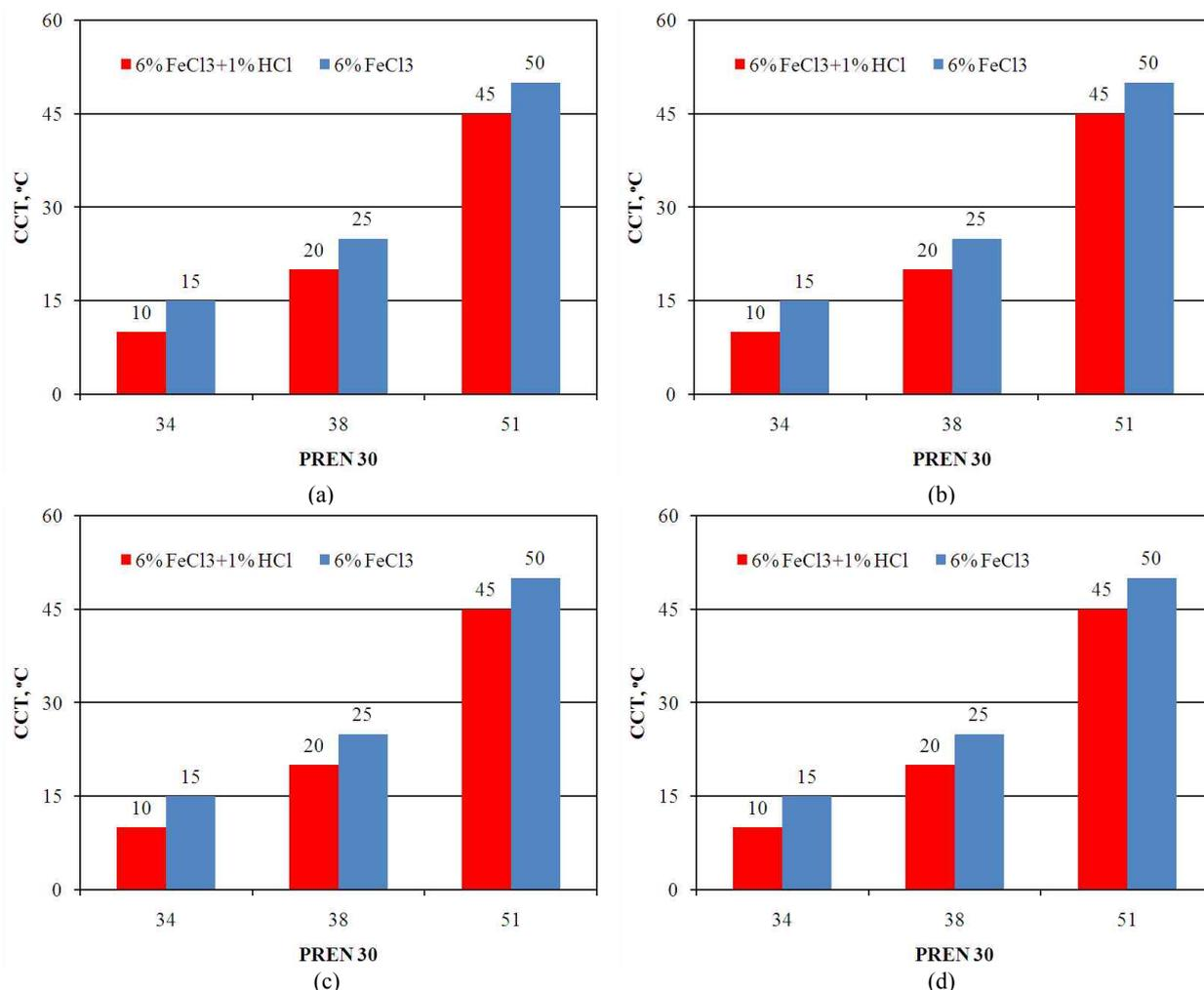
Fig. 9. CCT of the austenitic stainless steels determined in 6% FeCl<sub>3</sub> + 1% HCl and 6% FeCl<sub>3</sub> solution; (a) plate, and (b) round bar (D; 35 mm), (c) round bar (D; 25 mm), (d) round bar (D; 15 mm).
