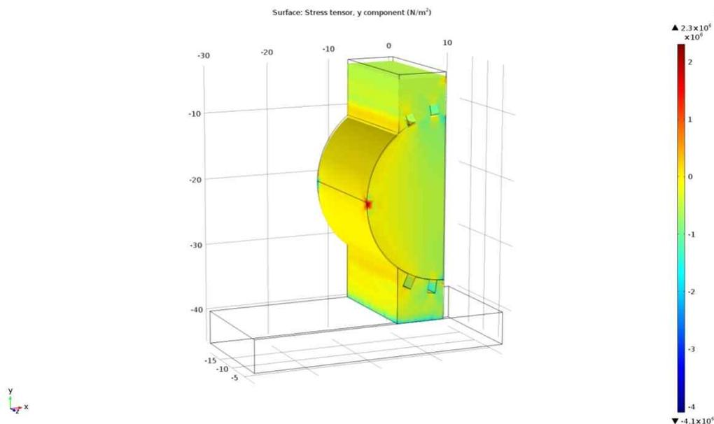
Fig. 12. Result of stress tensor (y component) distribution with strain (x-y-z). [symmetry model: torque 2.14 Nm(= vertical force 1103,9 N)].
