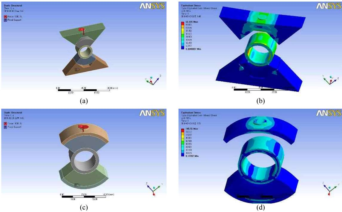
Fig. 2. Results of stress analysis for candidate designs of the crevice test assembly.
